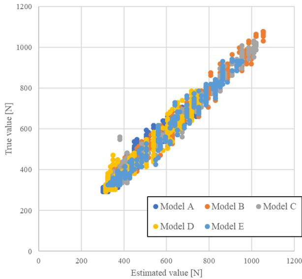
Figure 6. Comparison of disc compression forces estimated for untrained data by a deep learning model trained on an individual with the true values derived by AnyBody.
