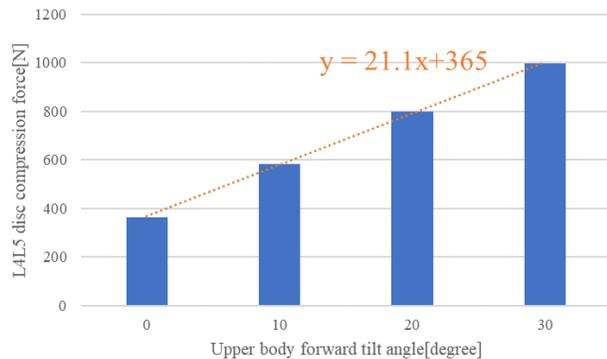
Figure 3. Compression force of intervertebral disc between L4/L5 derived using AnyBody for each angle of forward tilt of upper body.
