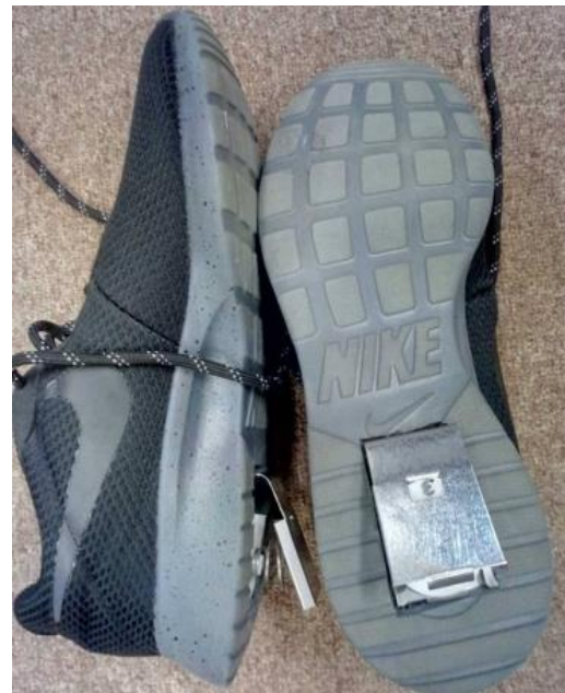
Figure 12. Pair of shoes with built-in spring assist units.
