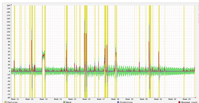
Fig. 2. Holt-Winters based vertical bands representing high occurrences of SSH login attempts resulting in "Failed password" messages.
