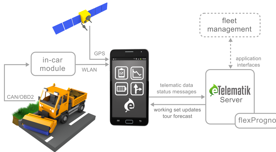
Fig. 1. eTelematik system architecture overview (adapted figure, based on original by Johannes Kretzschmar, University Jena)
