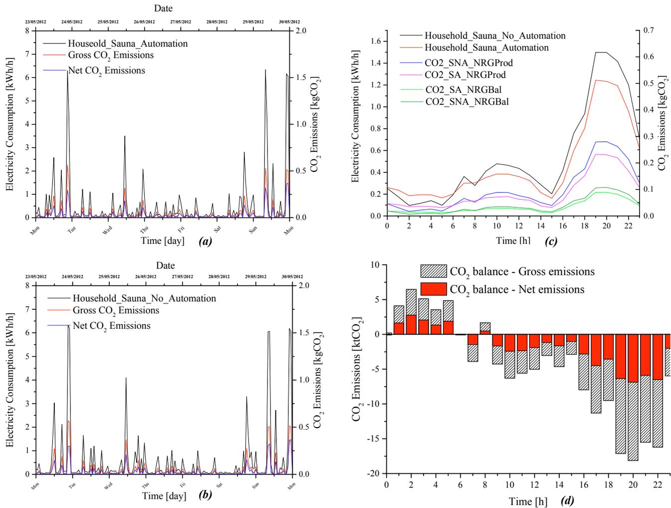
Figure 7. Electricity consumption with its related CO<sub>2</sub> emissions for (a) a dwelling with automation and (b) a dwelling without automation, (c) Daily electricity consumption profiles and (d) the related CO<sub>2</sub> emissions balance between both houses in terms of gross and net emissions
