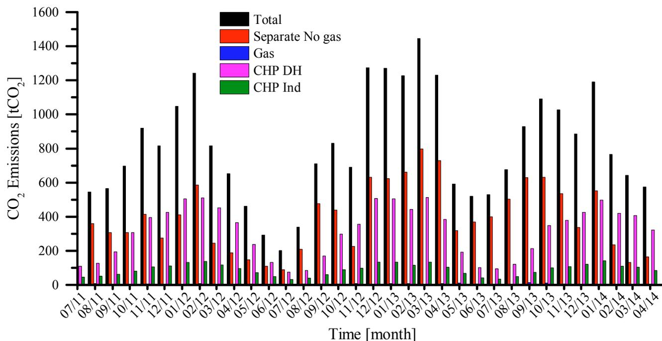
Figure 3. CO<sub>2</sub> emissions in Finland from conventional thermal power plants excluding gas engines, gas power plants, CHP from district heating and CHP from industrial electricity production, based on [32].
