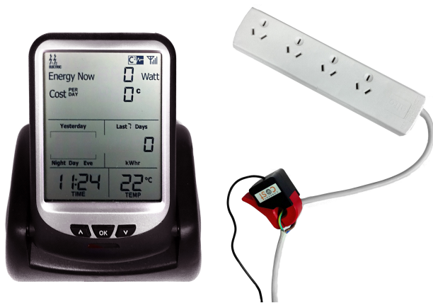
Figure 4: Current Cost base station (left) and jaw connected to a power-board (right).
