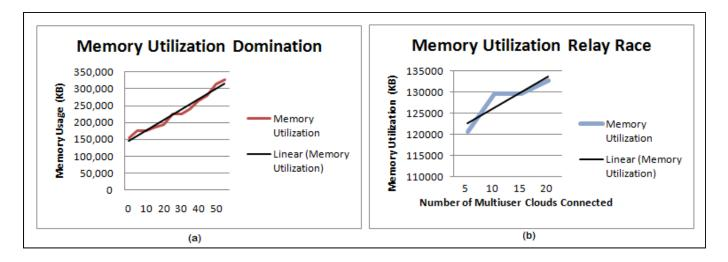
Figure 7: Memory Utilization (a) Domination Memory Utilization (b) Relay Race Memory Utilization
