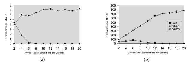
Figure. 8: Throughputs of long transactions (a) and small transactions (b) when heavy-tailed workload is used.
