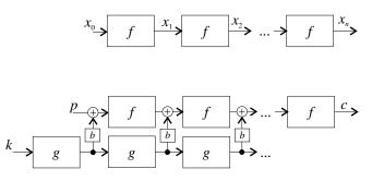
Figure 9. A typical block cipher which is a combination of several pseudochaotic systems.
