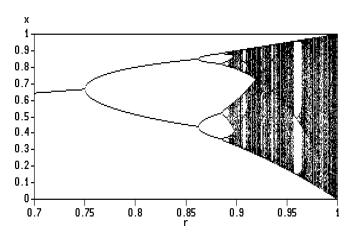
Figure 7. Bifurcation of the logistic map. The most 'unpredictable' behavior occurs when  $r \rightarrow 1$ .
