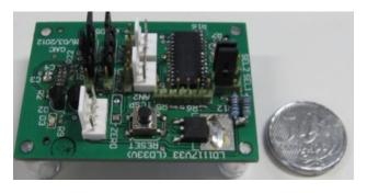
Figure 4. Intelligent Sensor Module (ISM).
