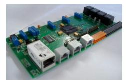
Figure 6. Remote Data Acquisition Unit (RDAU).
