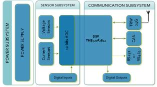
Figure 5. Remote Data Acquisition Unit (RDAU) Diagram.
