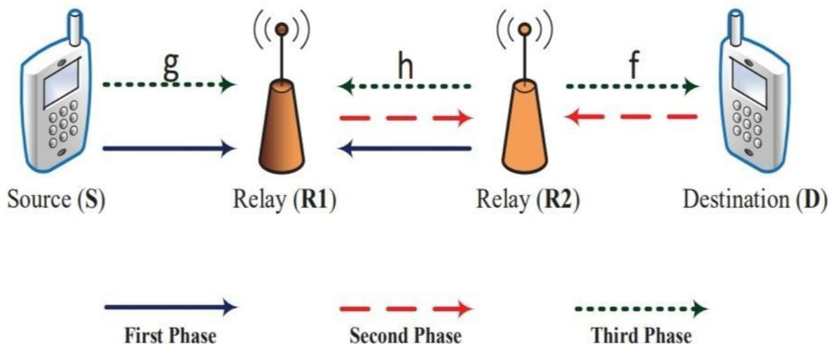
Figure 1. System model of a three-hop wireless relay [6].
