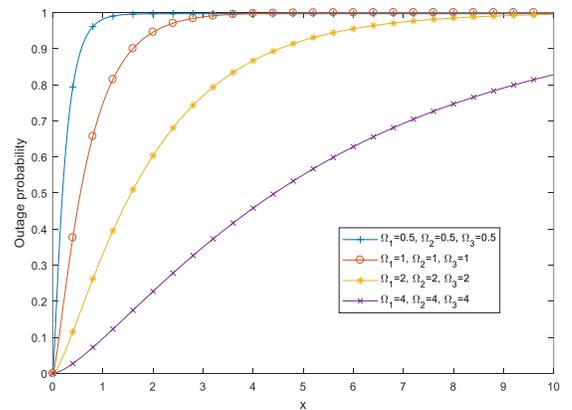
Figure 3. Outage probability of product of three Rician RVs depending on signal envelope for different values of signal power  $\Omega_i$  and Rician factor  $\kappa=1$ .
