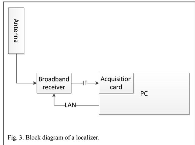
The localizer has been made in the technology of Software Defined Radio [7]. It consists of: an antenna, a broadband receiver, an analog to digital converter (in the form of data acquisition card) and a digital signal processor (in form of PC). This approach allows to shape flexibly functionality of the localizer.
