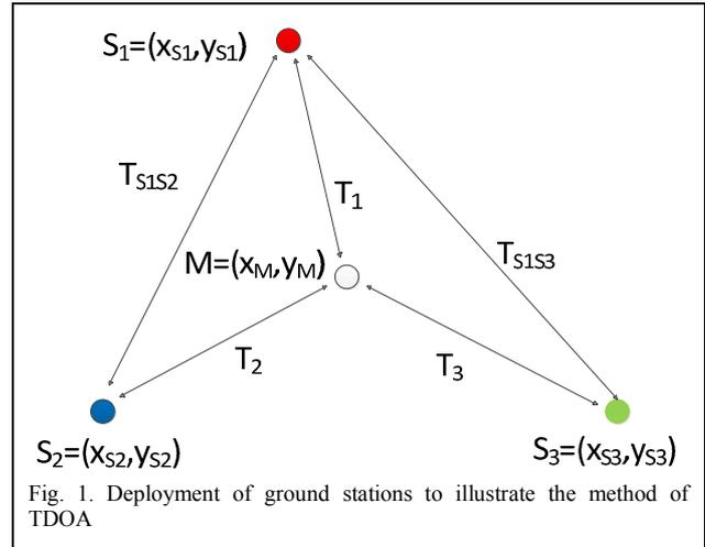
Fig. 1. Deployment of ground stations to illustrate the method of TDOA
