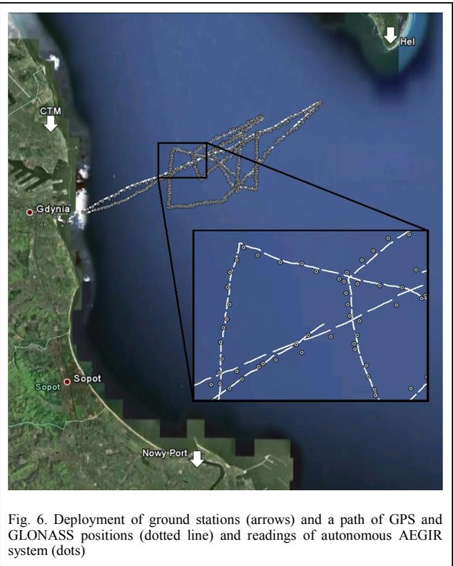
Fig. 6. Deployment of ground stations (arrows) and a path of GPS and GLONASS positions (dotted line) and readings of autonomous AEGIR system (dots)
