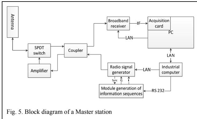
Fig. 5. Block diagram of a Master station
