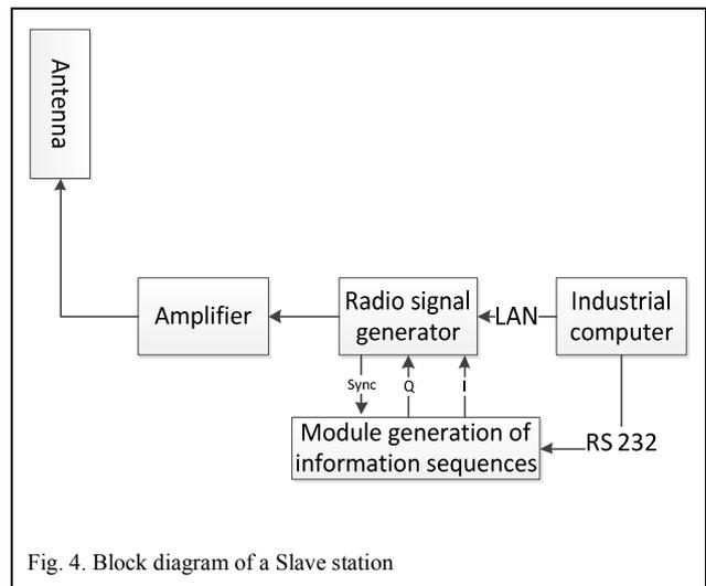
The main element of the station is a radio signal generator, whose task is to broadcast modulated signal with data that are generated by industrial computer.
