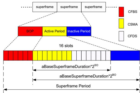
Figure 1. ADCF superframe structure.
