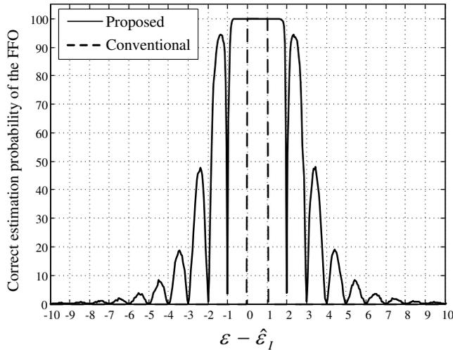
Figure 4. Correct estimation probabilities of the FFO as a function of  $\varepsilon - \hat{\varepsilon}_I$  for the proposed and conventional schemes in the Rayleigh fading channel model when G-SNR is 25 dB.
