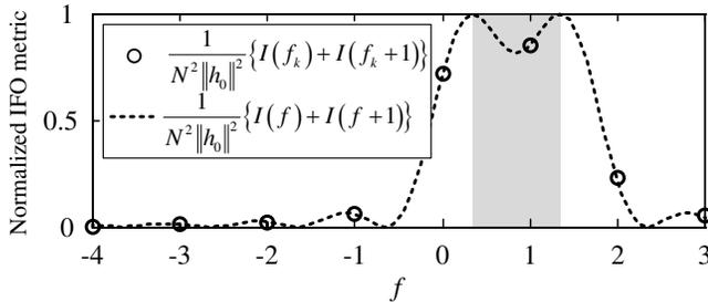
Figure 2. IFO metric  $\{I(f) + I(f+1)\}$  normalized to  $N^2 \|h_0\|^2$  as a function of the frequency  $f \in [-N/2, N/2]$  for  $\epsilon_F = 0.3$  when  $\epsilon_I = 1$ ,  $N = 8$ , and the noise is absent.
