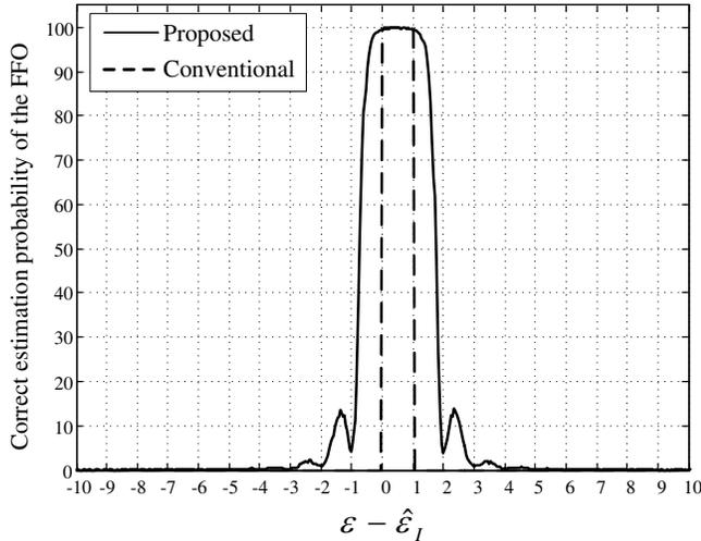
Figure 3. Correct estimation probabilities of the FFO as a function of  $\varepsilon - \hat{\varepsilon}_I$  for the proposed and conventional schemes in the Rayleigh fading channel model when G-SNR is 5 dB.
