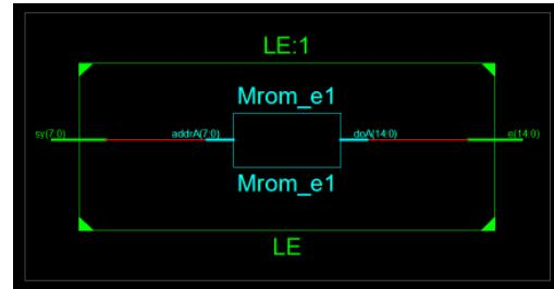
Figure 9. Register Transfer Level of LE unit
