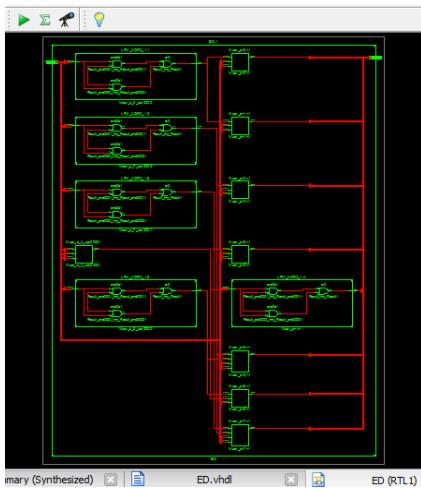
Figure 7. Register Transfer Level of the ED unit
