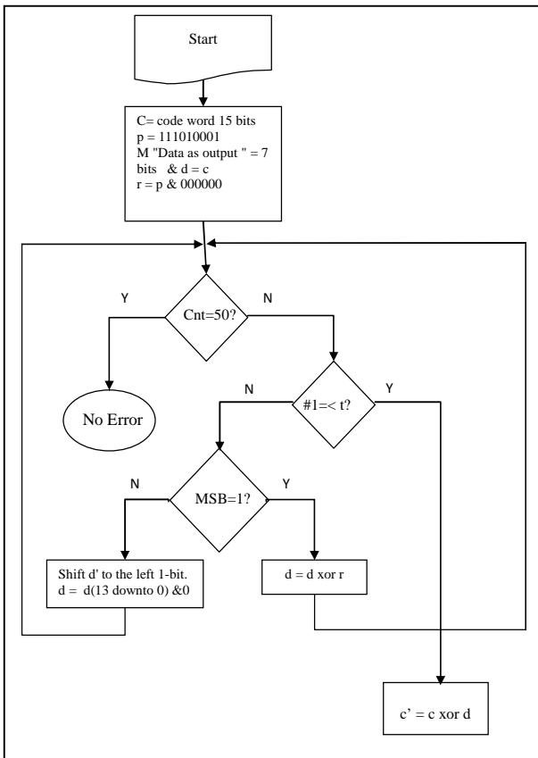
Figure 3. SM chart for a Modified CRC Decoding algorithm
