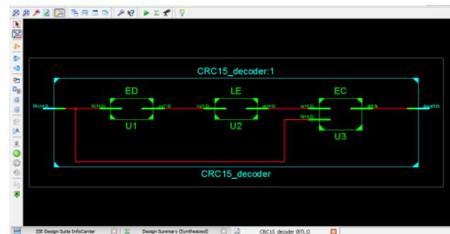
Figure 5. Second-level design of the decoder circuit
