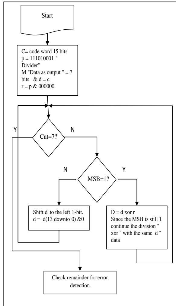
Figure 2. SM chart for CRC Decoding algorithm
