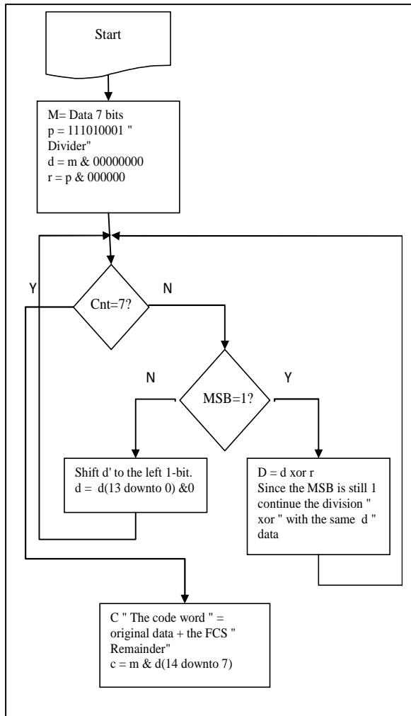
Figure 1. SM chart for CRC Encoding algorithm
