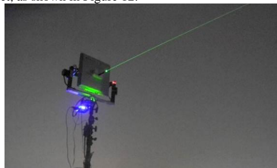
Figure 12. Stepper motor platform calibration with laser.
