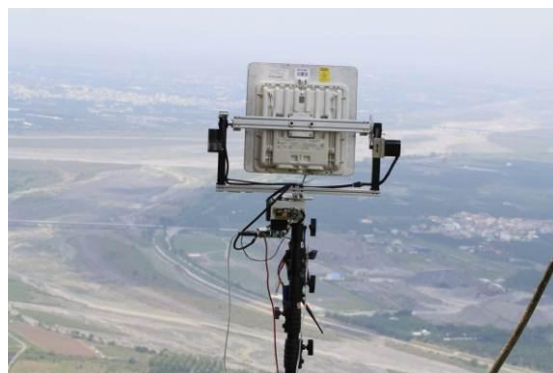
Figure 11. Ground terminal tracking unit with microwave module.
