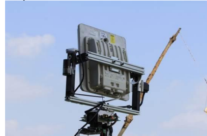
Figure 5. Two-axis Stepper Motor Rotation Platform.
