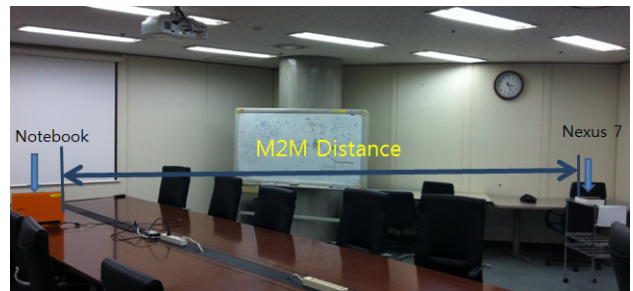
Figure 5. Bluetooth RSSI measurement test in meeting room environment
