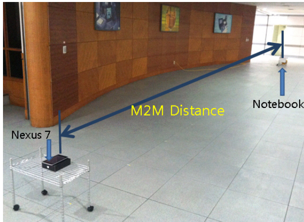
Figure 3. Bluetooth RSSI measurement test in indoor hall environment
