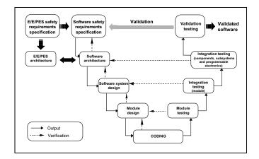
Figure 1. The V model of IEC 61508
