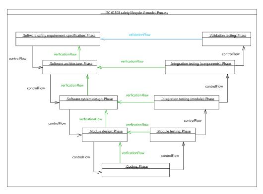
Figure 10. PPFS Metamodel instantiated by the IEC 61508 safety lifecycle.
