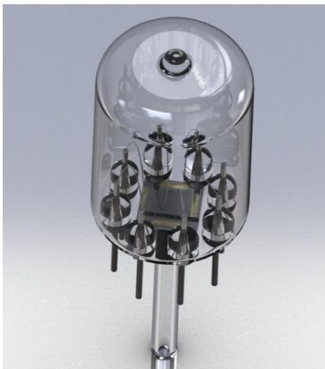
Figure 10. Possible package for emitter made from carbon nanotubes.
