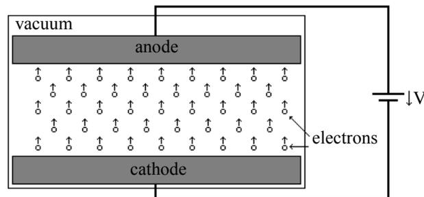
Figure 2. Schematic illustration and principle of measuring the emission properties.
