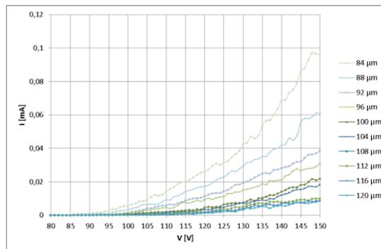
Figure 7. The detail result of measured emission current in dependence on the applied voltage for higher voltages.
