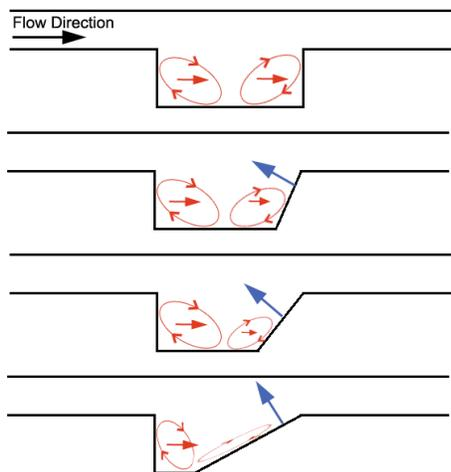
Figure 4. Geometry effects on the focusing mechanism
