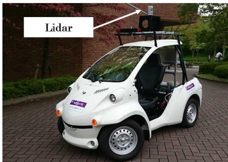
Figure 1. Overview of the experimental vehicle.
