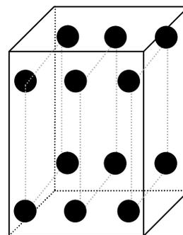
Figure 1. Distribution of nodes in the space of the cold chamber.
