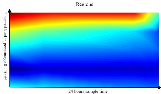
Figure 4. Distribution of the energy inside the cold chamber with different thermal loads.
