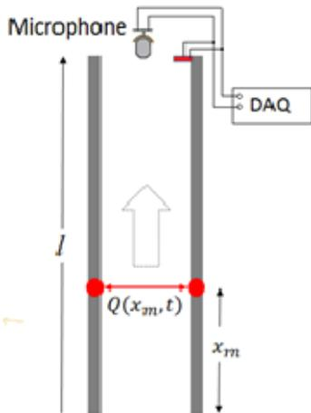
Figure 2. Data adquisition for Rijke tube experiment.
