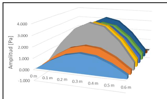
Figure 5. Fundamental mode of vibration in air column.
