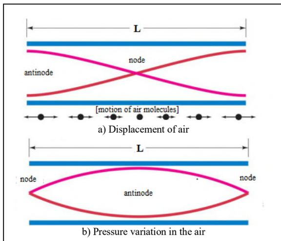
Figure 1. Pressure and displacement for the air in the columns.
