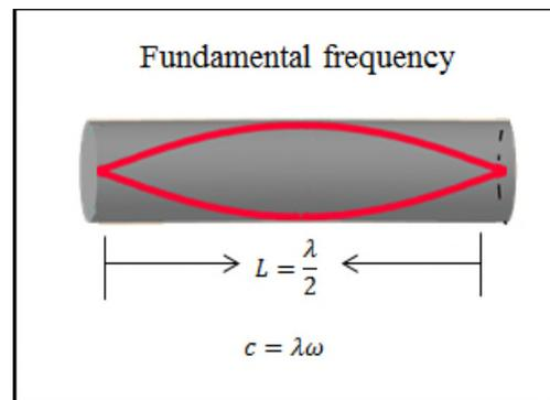
Figure 4. First vibration mode in air column.
