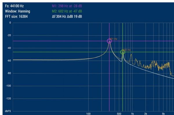
Figure 6. Fundamental frequency measure on Rijke tube experiment.
