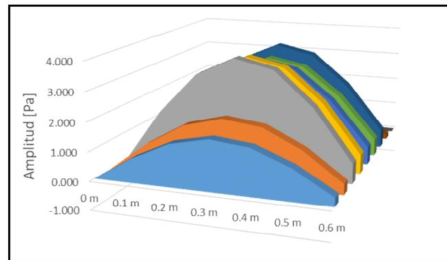
Figure 5. Fundamental mode of vibration in air column.
