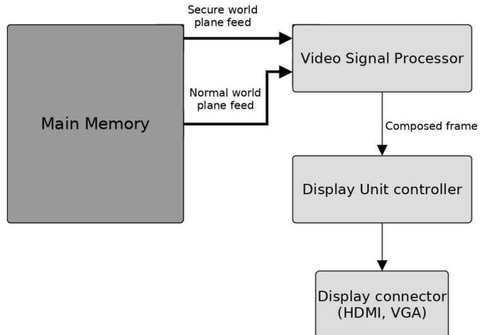
Figure 5. Hardware peripherals involved in the graphics pipeline
