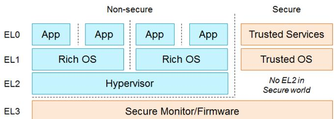
Figure 1. ARMv8 processor architecture [12]
