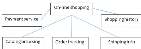
Figure 3. Example of microservice architecture
