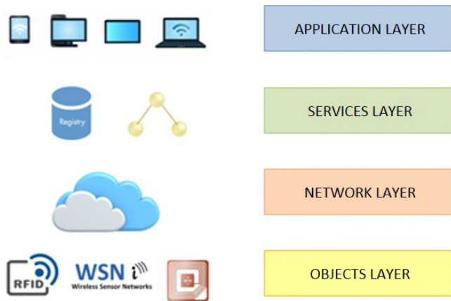
Figure 1. Architecture based on SOA for IoT systems.
