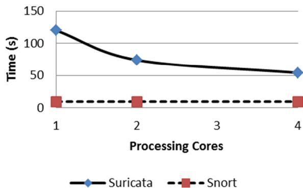
Figure 9 Pcap processing time (offline mode)
