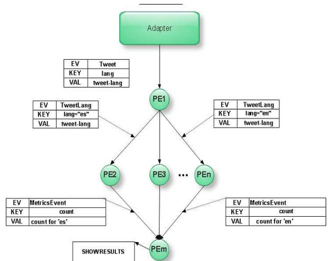
Figure 1. S4 application design (lang-count example).
