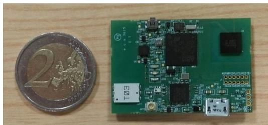
Figure 1. Tyndall Wireless Inertial Measurement Unit (WIMU).
