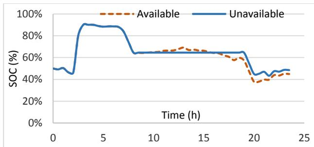
Figure 4. EV n°19 battery State of Charge (SOC) variation 2015/02/25.
