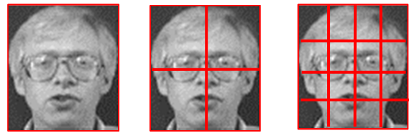
Figure 5. Image decomposition in different blocks.
