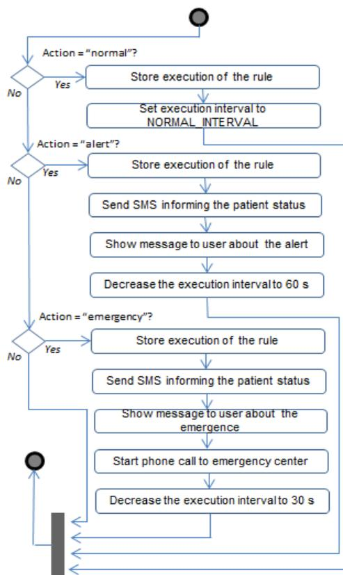
Figure 4. Activity diagram of the action control algorithm
