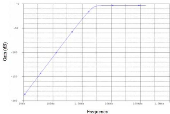
Figure 3. Simulated Frequency Response of Custom Filter
