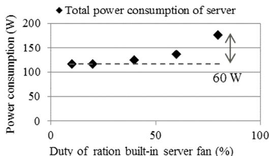
Figure 1. Power consumption of built-in server fan.
