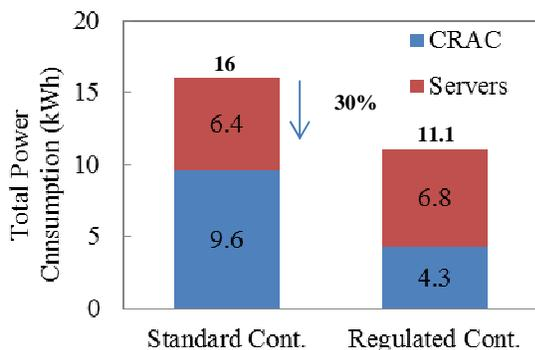
Figure 6. Comparison results of total power consumption
