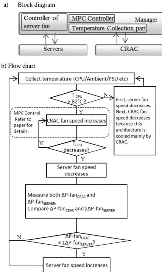
Figure 3. Block diagram of the proposed architecture.
