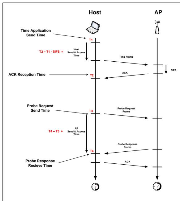
Figure 2. Determination of send and MAC delays
