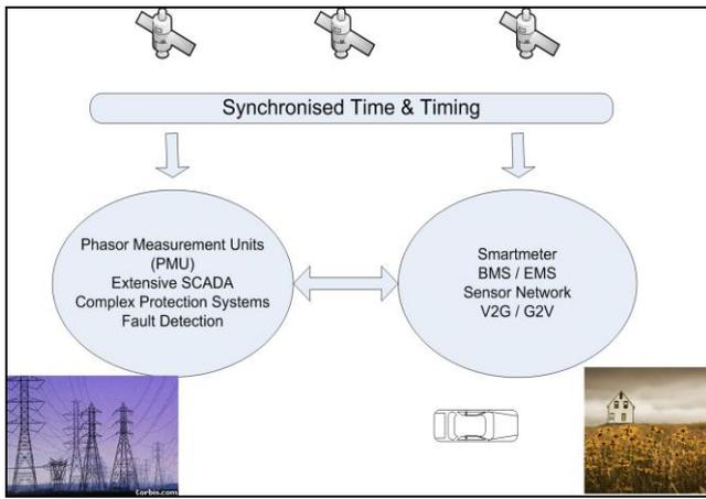
Figure 1- Synchronisation of Grid Elements
