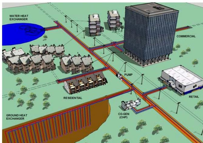
Figure 3. Example of geexchange system integrated with co-gen
