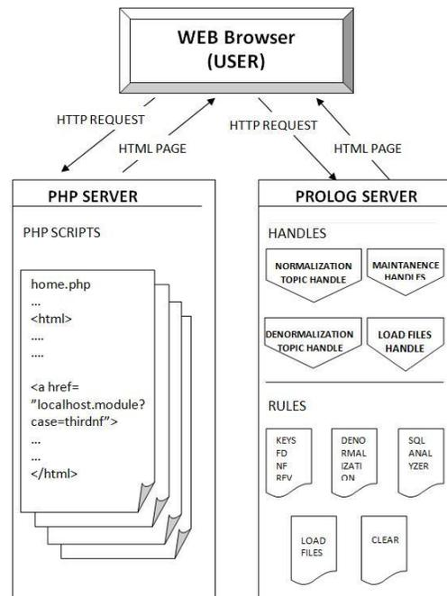
Figure 2. Workflow and request chains of NORMALDB tool.
