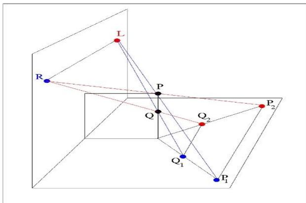
Figure 3. Horizontal plane projections of the P and Q points, according to the positions of the left eye (L) and right eye (R).
