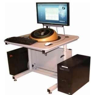
Figure 2. Maglev 200<sup>™</sup> Magnetic Levitation Haptics
