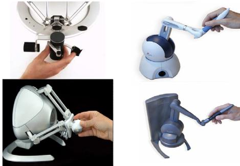
Figure 1. Omega.x (top-left), Falcon Novint<sup>™</sup> (bottom-left), PHANTOM<sup>™</sup> Omni (top-right) and Desktop (bottom-right)
