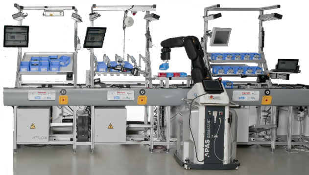
Figure 1. Assembly system with manual and human robot collaboration workstations.
