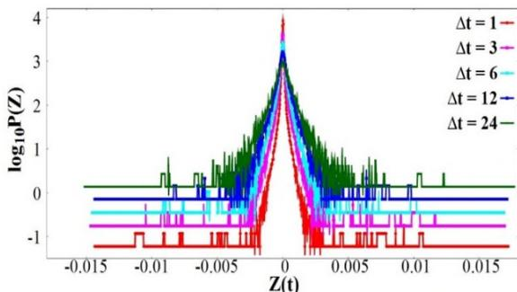
Fig.1 The histograms of statistical distribution of Z for  $\Delta t=1$  (5 sec), 3 (15 sec), 6 (30 sec), 12 (1 min), and 24 (2 min).
