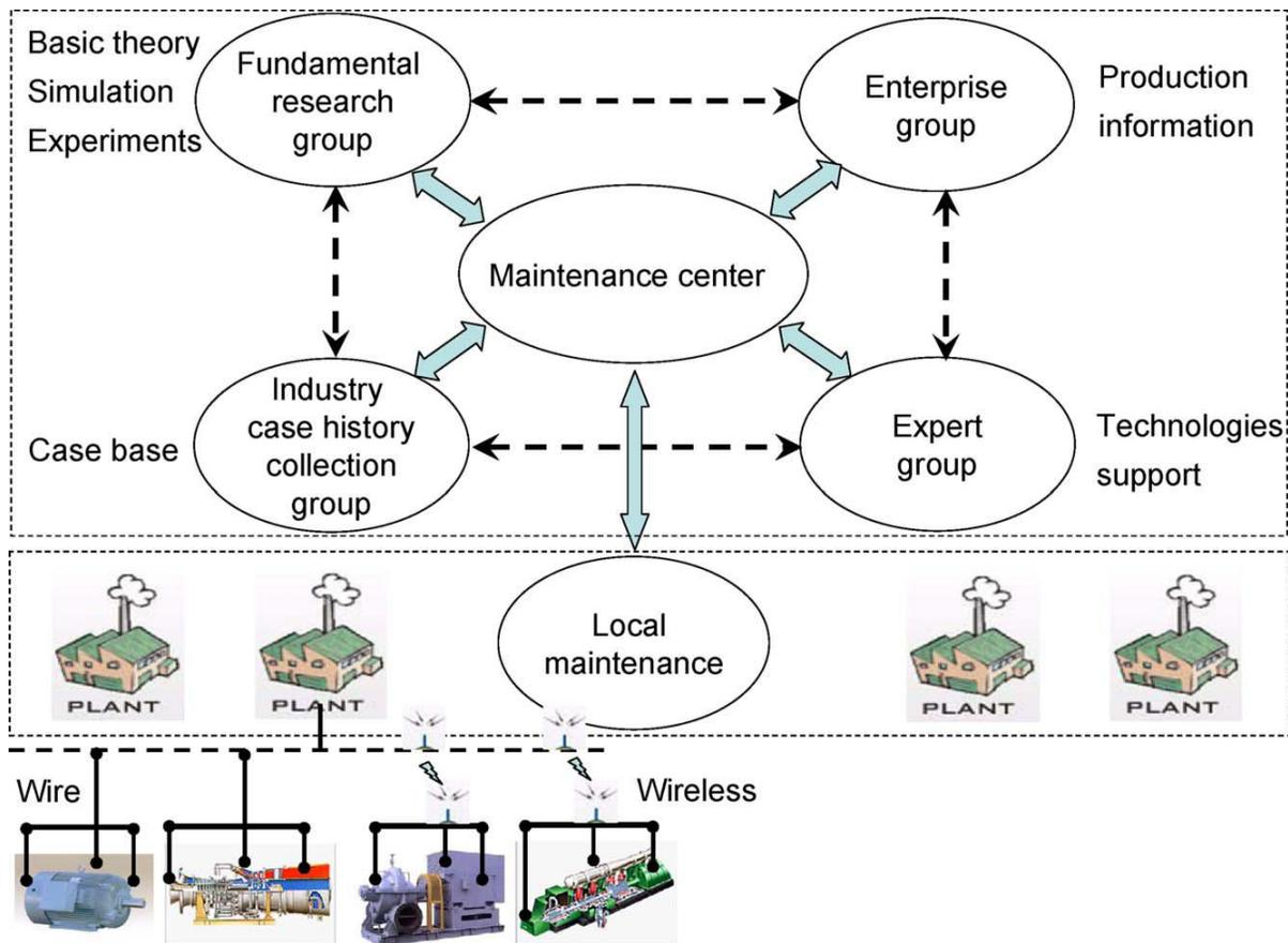
Figure 1 – Architecture of a hypothetical e-maintenance system; adopted from Han and Yang, 2006.
