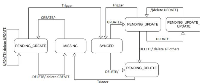
Figure 7. State machine of the change tracking mechanism.
