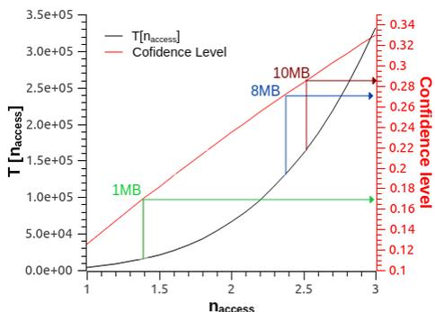
Figure 3. Confidence level required for filling of 32/4 PCache
