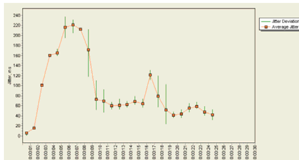
Figure 3. Measured jitter through the EDGE radio access network in the case of voice and video communication
