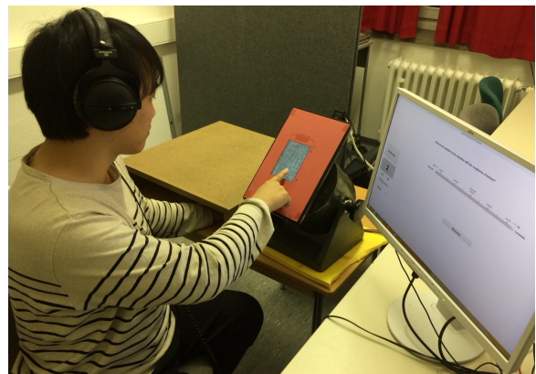
Figure 2. The experimental setup and the evaluation interface are seen above. During the evaluation, the participants touched the sand papers under the wood cover.
