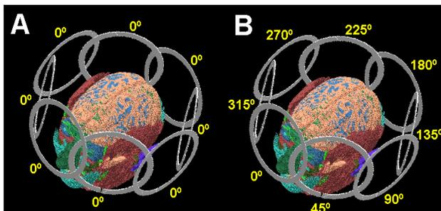
**Fig. 2** (Left) Geometrical model of the coil array and our model [13] with examples of null (A) and uniform (B)  $\vec{q}$  vectors [17]. (Right) 8-channel transmit phase array FDTD  $B_1$  maps (nT/ampere) of the center transverse slice of our model when each channel is driven with a 1-ampere peak-to-peak 300-MHz sinusoid [18].
