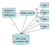
Figure 3. The architecture of MRlite
