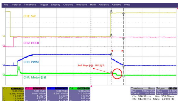
Figure 8. Measured motor control signal and current profile generated by control of voltage to DC motor with the developed motor driver.
