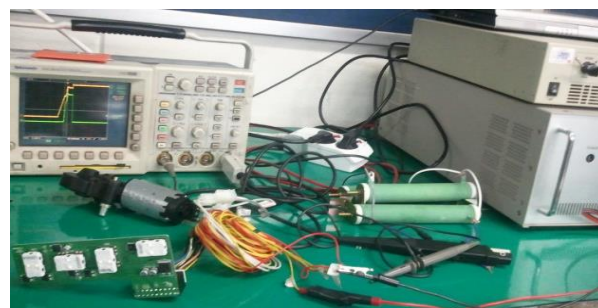
Figure 6. Experimental setup for the performance test of developed DC motor driver.
