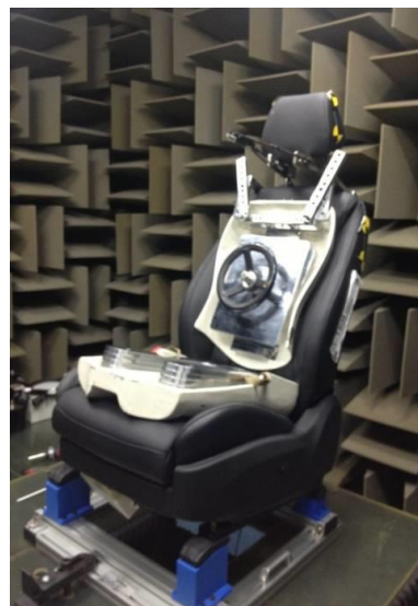
Figure 9. Experimental setup for the performance test of seat motion by applying the proposed control method in the dead sound chamber.
