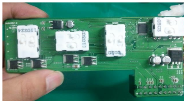
Figure 5. Developed DC motor driver having the functions of soft-start and soft-stop.
