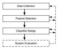
Fig. 3. Design stages of a pattern recognition system
