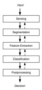
Fig. 9. The components of a typical pattern recognition system [9]
